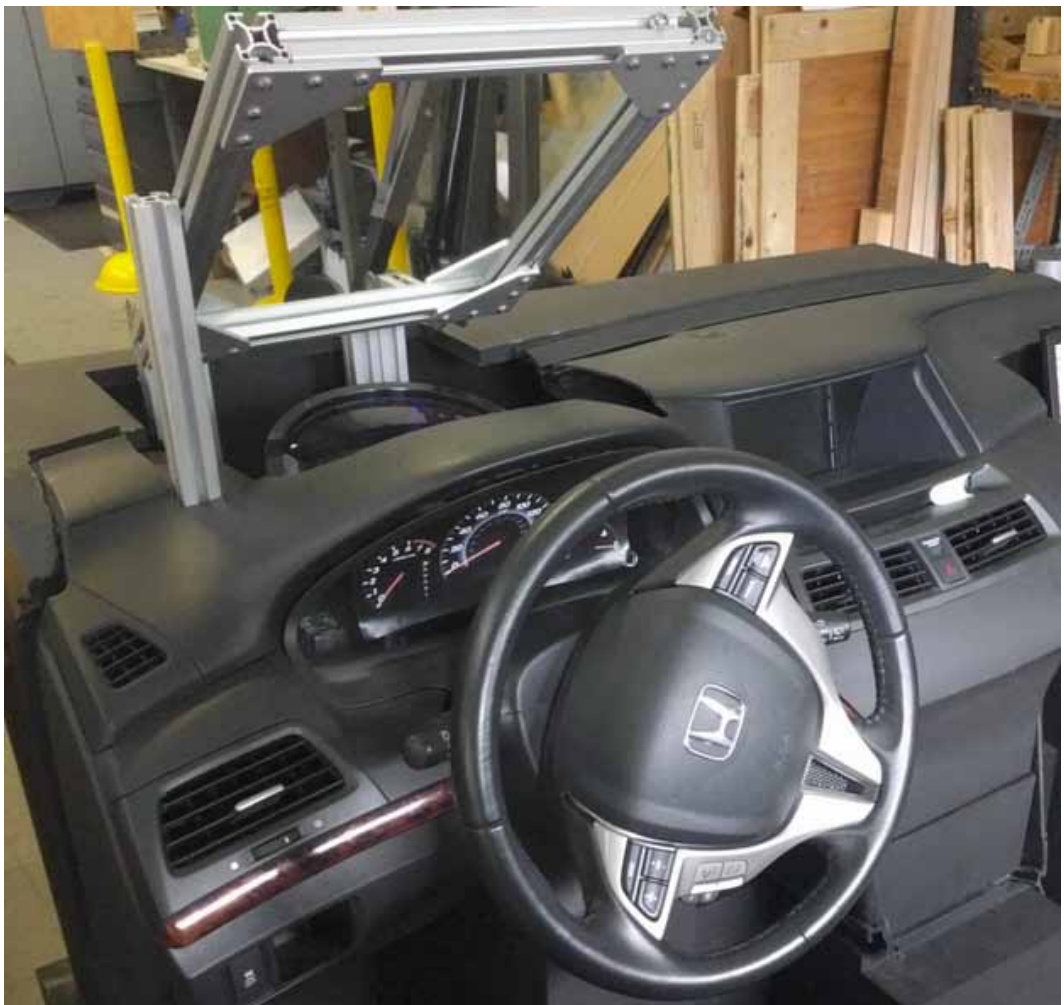
Figure 2. The volumetric AR display used in our experiment was housed in a fixed mockup vehicle dash. Participants viewed the virtual rectangles and real-world referents through the glass pane located above the steering wheel.
