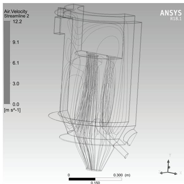
Fig. 4. Streamline of air and biomass in boot device
