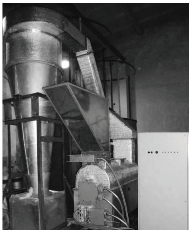
Fig. 5. Experimental installation with an automated control system for plant biomass destructive energy processing
