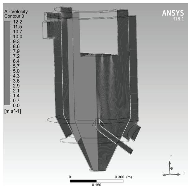
Fig. 3. Air velocity distribution in boot device
