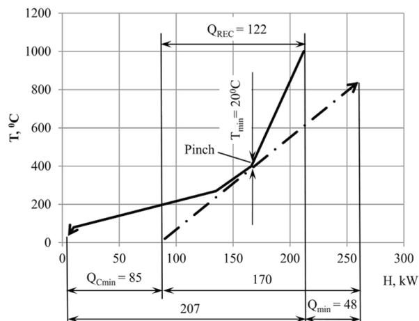
Fig. 2. Heat exchange of cold and hot streams, internal and external heat exchanging surfaces of active parts
