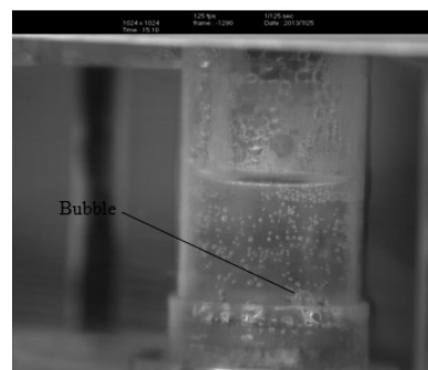
Fig. 13 Formation of bubbles in compensation chamber
