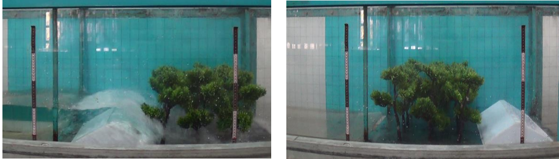
Figure 1- Tree-structure arrangement in the laboratory flume
