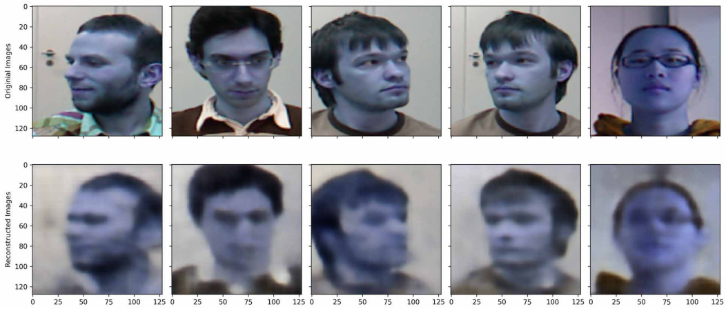
Figure 8. Original and reconstructed faces using a VAE
