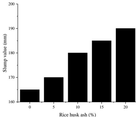
**Figure 6.** Effect of rice husk ash on slump
