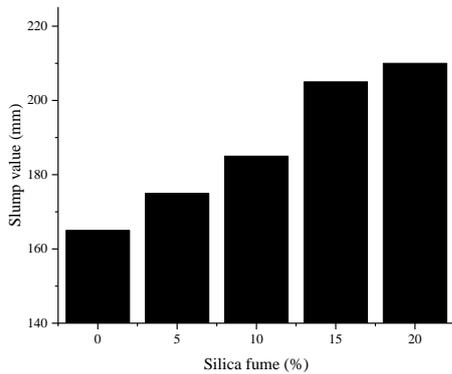
**Figure 5.** Effect of silica fume on slump
