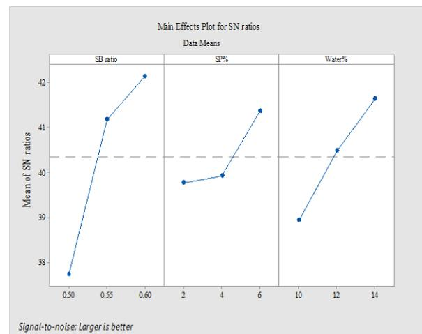
**Figure 2.** Main effects plot of SN ratios for slump
