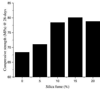
**Figure 7.** Effect of silica fume on Compressive strength
