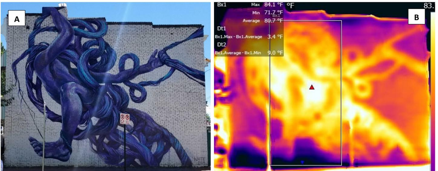
**Figure 3.** North wall art mural (A) and its corresponding thermal emittance image (B) indicating maximum, minimum, and average thermal emittance temperatures at 1444 hours EDT (Lux = 9000), 09 July, 2018. Maximum and minimum readings were taken within a fixed grid to control extraneous factors (e.g. windows, asphalt, skies) that would skew temperature readings.
