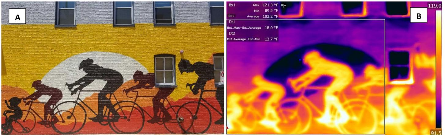
**Figure 2.** South wall art mural (A) and its corresponding thermal emittance image (B) indicating maximum, minimum, and average thermal emittance temperatures at 1305 hours EDT (Lux = 36000) 18 July, 2018. Maximum and minimum readings were taken within a fixed grid to control extraneous factors (e.g. windows, asphalt, skies) that would skew temperature readings.
