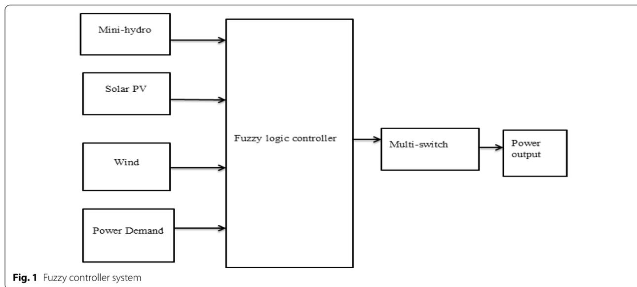
in MATLAB toolbox. These rules are loaded on the fuzzy logic controller for controlling the hybrid power system. Varying load demand of the community is switched to the available source according to written Hailemariam et al. (2015).
