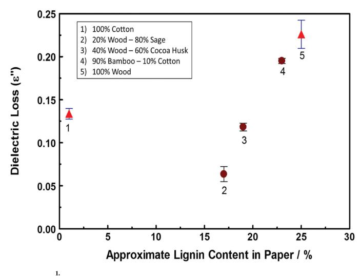
Dependence of dielectric loss profiles (slope, see Eq. 1) on estimated weighted lignin fraction in the analyte. The weighted lignin fraction was calculated from the average literature values of lignin content in each fiber source weighted for the advertised composition.
