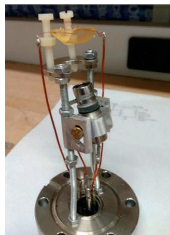
**Figure 13.** Homemade channeltron and Golden Woven Mesh holder lodged in a feedthrough flange (maximum current 10 A) for the vacuum chamber.
